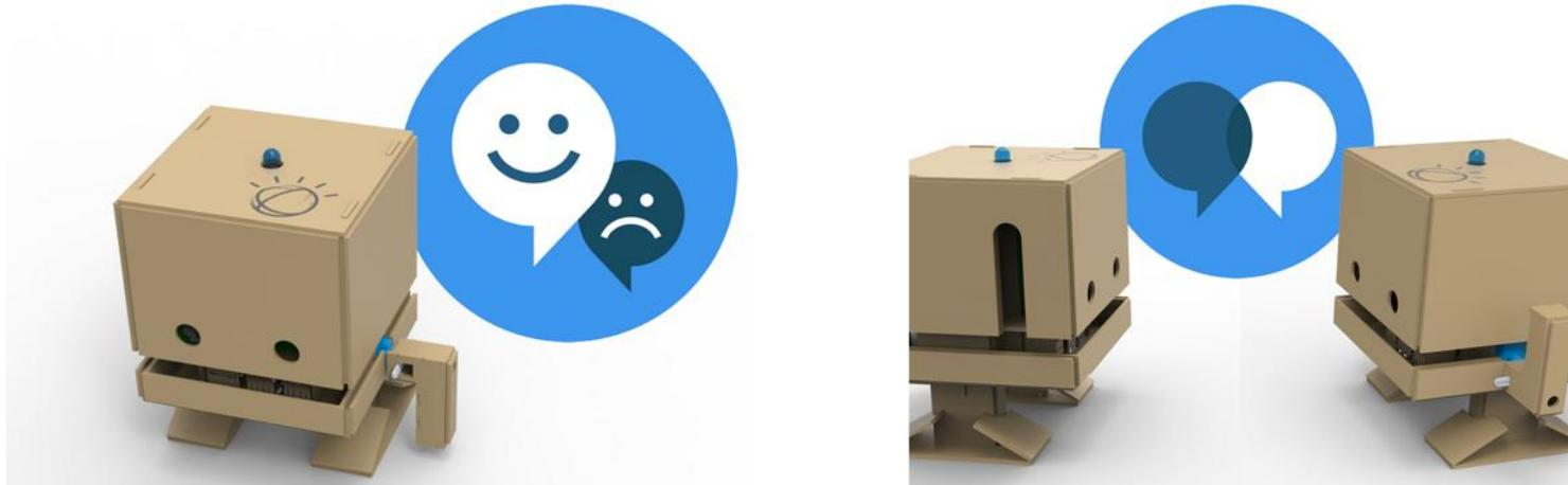
**Hardware:** Raspberry Pi, Camera, Servo Motor, Speakers, Microphone, SenseHat (optional)
